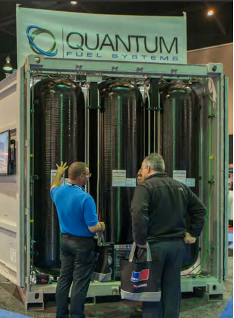
Quantum Fuel Systems , which has the highest capacity gaseous trailers in the industry, displayed a section of their Virtual Pipeline Trailer for CNG transport, as well as their back-of-cab CNG fuel system for class-8 trucks.
