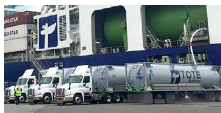
TOTE – LNG-Powered Container Ship and On-Dock ISO-Tank LNG Bunkering
